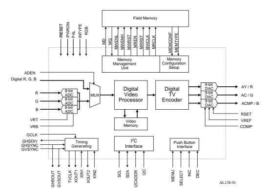
An integrated high-quality anti-flicker filter (SmartFilter<sup>TM</sup>) removes the unpleasant flicker caused by the interlaced display of high contrast graphics while maintaining the original clarity and sharpness of informative data such as natural pictures and text.
